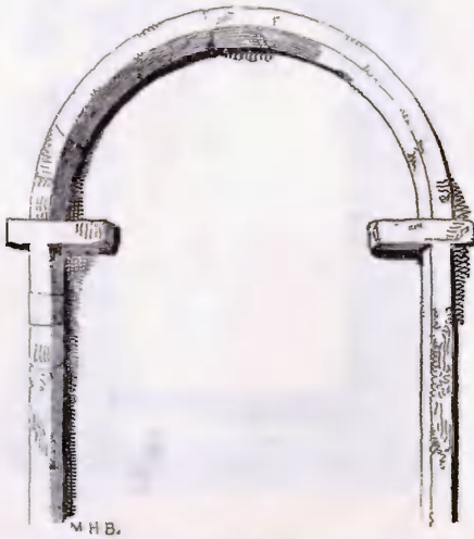
Pilaster Rib-work Arch, Brigstock Church.
